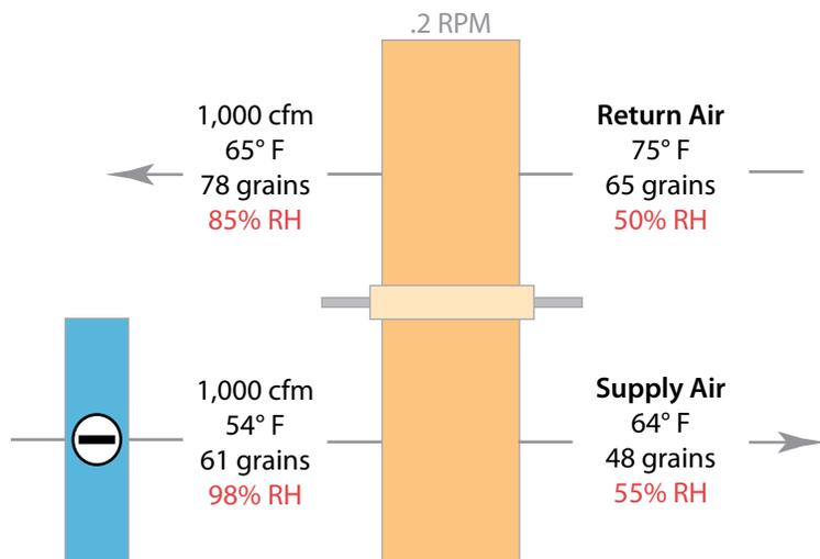
Aside from these differences, the passive and active desiccant wheels perform the same function and are driven by the same thermodynamic principles. The obvious advantage of the passive wheel is that no regeneration energy is required. The advantage of the active wheel is that the high regeneration energy allows for more moisture to be removed (greater grain depression).
