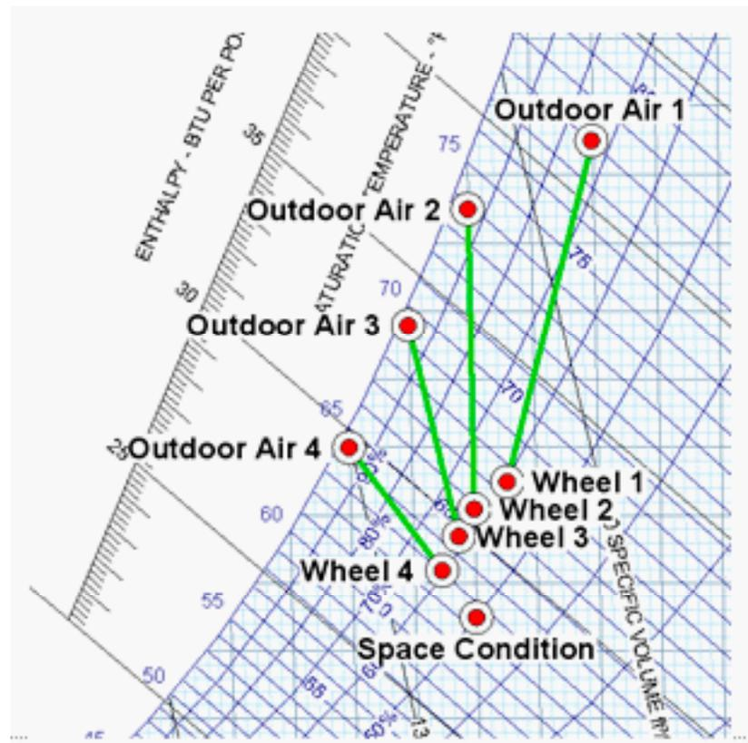
Figure 6 is provided to show various outdoor air conditions that frequently occur during the cooling and dehumidification seasons. It assumes that the space is conditioned to 75°F at 50% RH and that this condition is exhausted from the building. An 81% effective total energy wheel processing 10% more supply airflow than exhaust is used.
