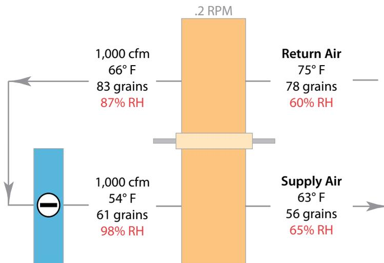
Figure 5. Sample “wrap around” passive desiccant wheel performance.
