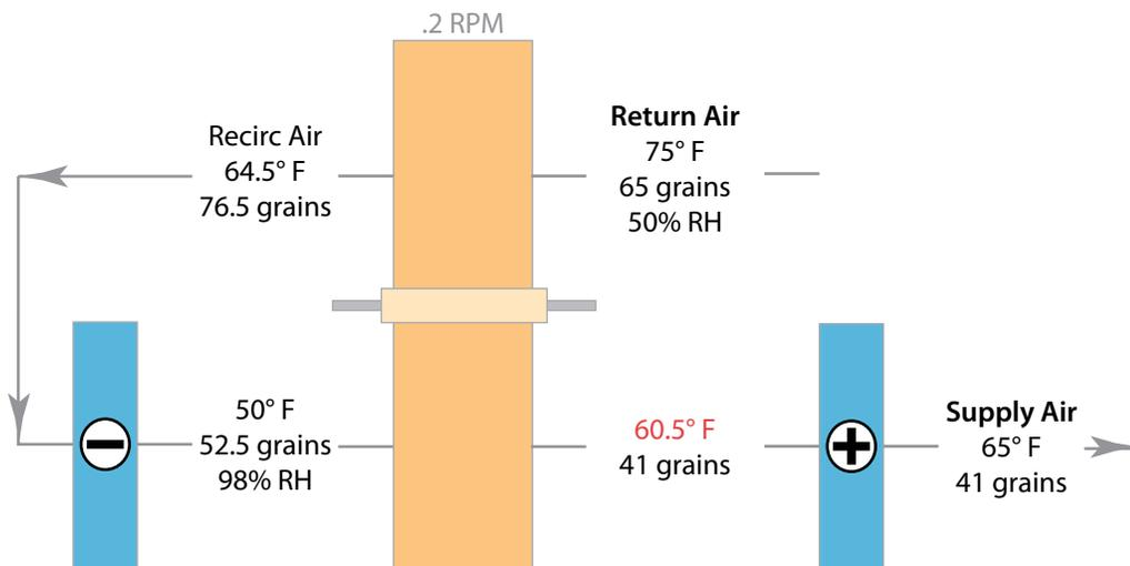
Figure 4. PD wheel not modulated - parasitic reheat energy required.
