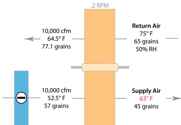
Figure 2. Sample SEMCO passive desiccant wheel - less reheat.
