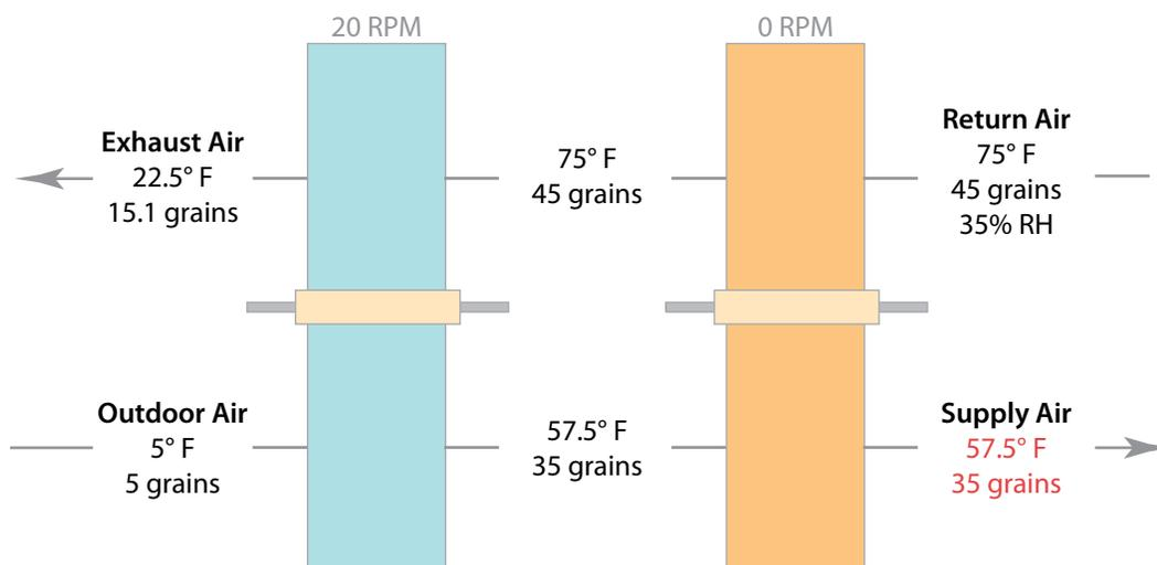
Figure 6: PD wheel off - far less recovery provided.
