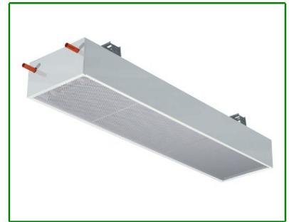
The Flexicool® QPVA and QPBA passive chilled beams provide for the cooling in a room. QPVA (width 570 mm) and QPBA (width 430 mm) are broad passive chilled beams. The passive chilled beams are either ceiling installed, in which case they lie flush with the suspended ceiling, or free space installed without ceiling.
