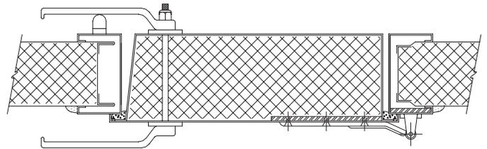
Pre-hung access doors are designed as an integral part of the panel system. Each door is provided with a minimum of two KASON 1061 hinges and FläktGroup SEMCO door latches operable from both sides of the door.
