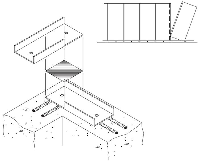
Panels are slipped into the base channel and secured with self-tapping sheet metal screws at the base channel to maintain plumb - screws at the joints are NOT required.
