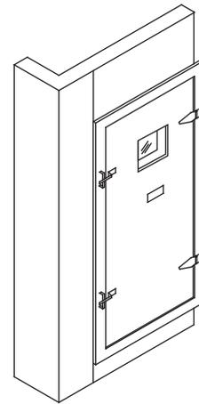
Access doors are supplied pre-hung with all hardware factory installed.
