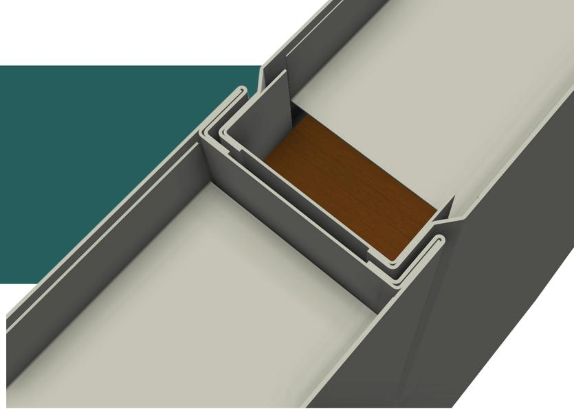
The integrity of the panel joint determines the overall performance of the AT-PANEL Acoustic/Thermal Panel System. Panels must be airtight [leakage rate of less than one half percent (<0.5%)], acoustically sound, rigid, and still be cost-effective during installation. Below are details of the different types of commercially-available panel joints.
