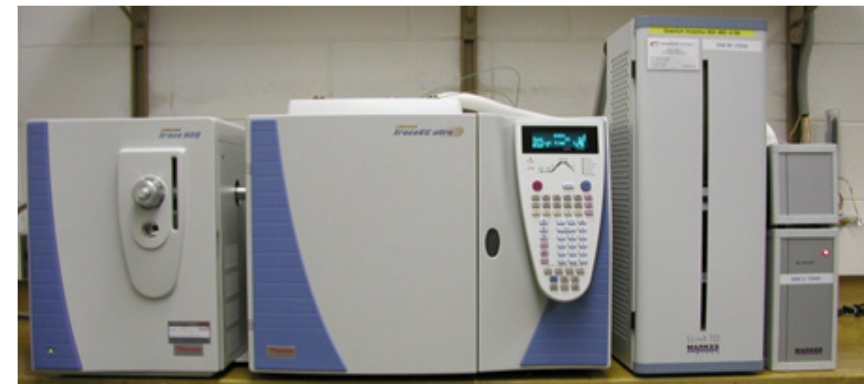
FIGURE 5. Gas chromatograph/mass spectrometer used to analyze TVOC samples
