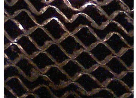
FIGURE 5: Ten times magnification of core 1, the untreated sample after the simulated 4 years of heavy ETS loading and compressed air cleaning. As compared to Figure 3, much of the buildup has been removed but approximately 30% still remains.
