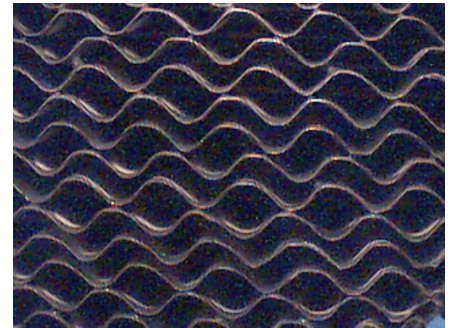
FIGURE 6: Ten times magnification of core 2, the anti-stick treated sample after the simulated 4 years of heavy ETS loading and compressed air cleaning. Essentially all the buildup observed in Figure 4 is removed.
