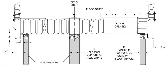
1. ROOF CURB SHOULD BE SIZED TO ALLOW UNIT TO HANG OVER CURB.
