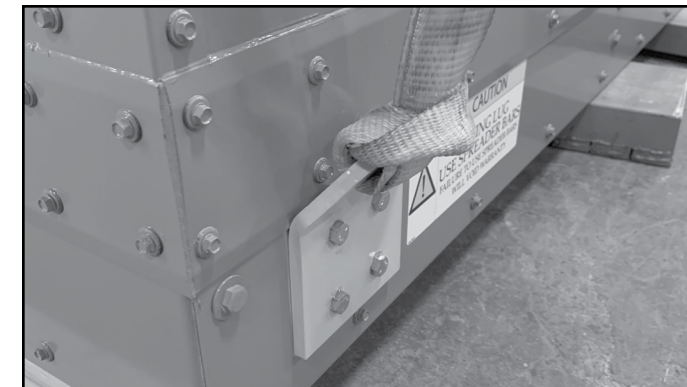
FIGURE 2. Lift modules only with lugs located at the base of each module. Do not use a forklift. NOTE: Chain hoists used to level unit.
