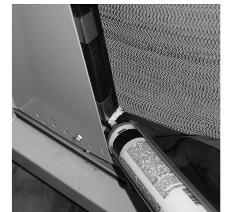
FIGURE 31. After adjusting the purge and tightening the adjusting and bottom pivot bolts, apply silicone caulk where the purge wiper joins the purge front plate.
