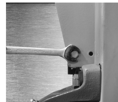
FIGURE 30. After removing the adjusting bolt(s), loosen the bottom pivot bolt.
