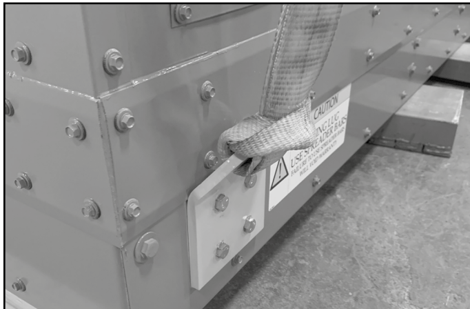
FIGURE 2 Lift units only with lugs located at the base of each unit. Do not use a forklift. NOTE: Chain hoists used to level unit.
