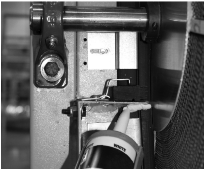
FIGURE 21. Caulk gap where purge seal abuts sheet metal end wall at the base of the purge.
