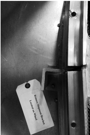
FIGURE 14. Shipping restraint for ribbed rim wheel.
