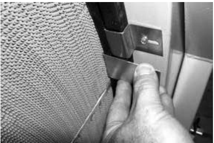
FIGURE 19. Loosen clip and insert gauge. Adjust seal to correct gauge depth.
