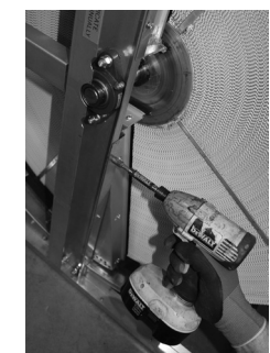
FIGURE 32. Remove screws from Sheet Metal Frame purge section.
