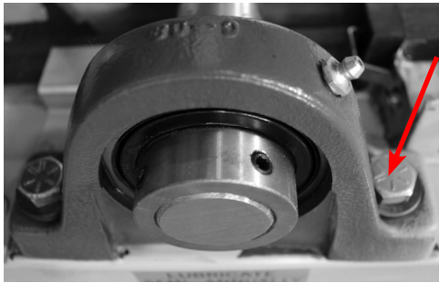
FIGURE 16. Inspect the bearing collar to ensure all bolts and screws are tight.
