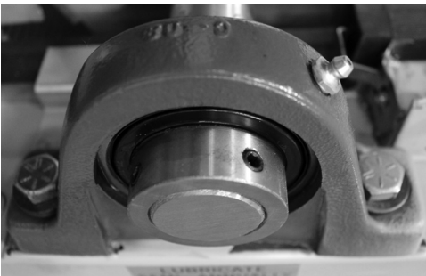
FIGURE 12. Pump grease into two rotor bearing grease points, one on each side of the rotor.
