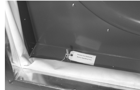
FIGURE 16. Two restraints in the fan inlet which bolt the fan to the base rail.
