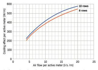
The diagram shows the total cooling effect per active metre at a total pressure of 70 Pa, water flow  $q_w = 0.05$  l/s , temperature difference between room air and supply air  $\Delta t = 8$  °C and temperature difference between mean water temperature and room temperature  $\Delta t = 8$  °C.
