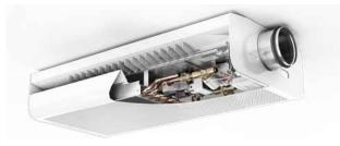
The room controller is factory mounted and wired on top of the front plate of NOVA II hidden from sight. In this configuration, the temperature sensor built into the room control tower is used. Temperature and condensation (in option) sensor are factory wired.
