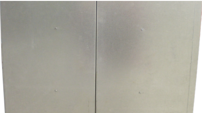
SAFE SIDE Two sides of the same panel after a two-hour, 1800°F flame test.
