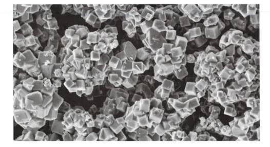
Figure 1: 3A Molecular sieve desiccant coating (SEM 10,000 x)
