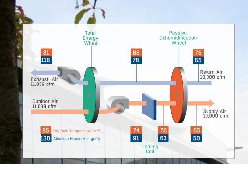
Schematic of the Pinnacle system operating at peak space latent load providing 89.5 tons of total cooling at a Sensible Heat Ratio (SHR) of 0.27 using only 51.4 tons of refrigeration input. The dew point delivered to space is 48.15°F. A conventional system with the same leaving coil temperature will NOT deliver the same dewpoint. It would require 97.4 tons of refrigeration and 226 MBtuh to achieve the same leaving coil condition.
